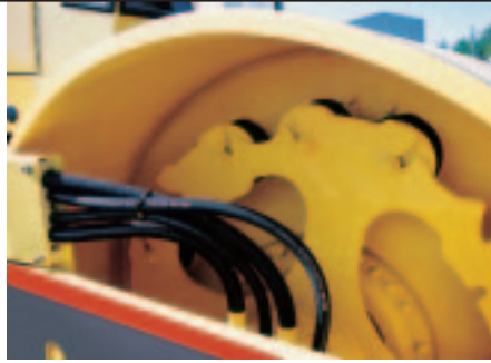
Individually changeable rubber buffers with no special tools or disassembly of the drum required
