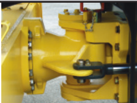
Maintenance-free, rugged, oscillating-articulation joint bolted on the outside of the front and rear frames
