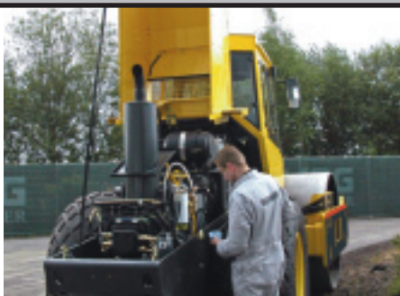
Large steel engine hood provides easy access to all service and maintenance points
