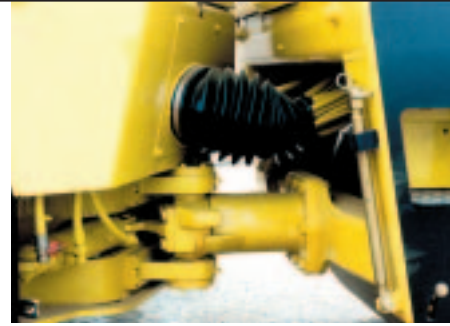
Bolt-on, maintenance free center joint provides high strength and long life. Excellent jobsite maneuverability is obtained through the articulation / oscillation provision.
