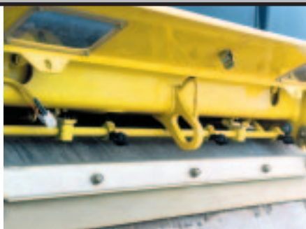
Non-corrosive, quick-disconnect, water spray nozzles are protected by a "flip-up", wind deflecting, spray shield.
