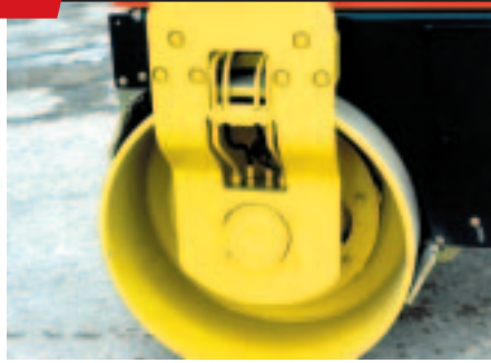
Leg design drum mounting provides high curb clearance, minimal lateral overhang and excellent drum edge visibility. Dual scrapers per drum are standard.
