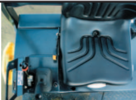
Laterally sliding seating position with controls. All critical controls are strategically positioned for ease of operation and safety.
