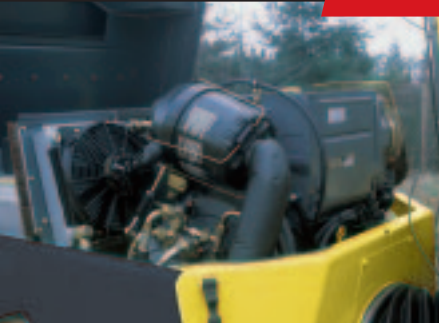
Field proven and reliable Deutz Diesel Engine with two (2) operating throttle positions, economy and performance.
