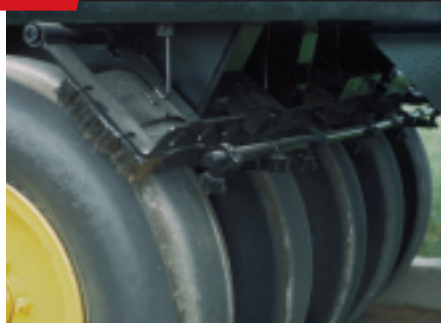
Standard equipped cocoa mats help to clean tires and minimize material pick-up
