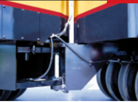
Maintenance free centerpoint articulation joint provides 35° steering angle and 10° frame oscillation
