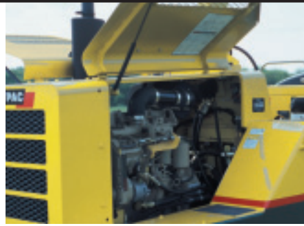
Wide, swing open doors provide quick and easy component access
