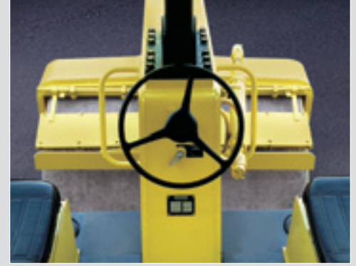
Dual operating seats provide an excellent view of the drum's edge
