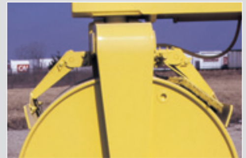
Each drum has a full width cocoa mat, two scrapper bars that clean in both travel directions, and five spray nozzles
