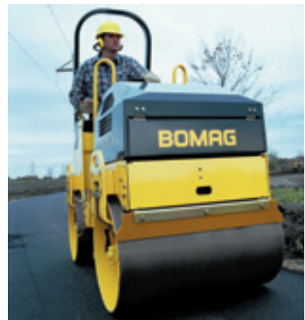
BW90AD-2 in action on an asphalt repair
