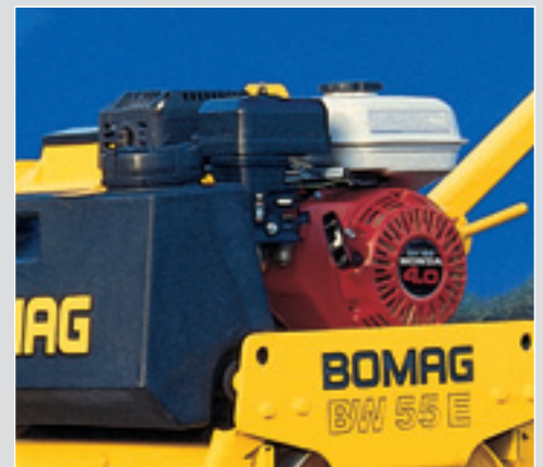
The BW55E is equipped with the 3.0 hp Honda engine
