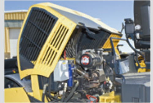
Easy opening, single hood, allows service with your feet on the ground.
