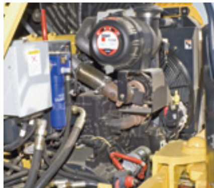
The engine is placed low in the frame for ease of service and operator visibility
