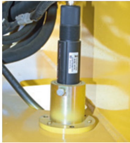
The Asphalt Mat Temperature Sensing System's on-the-go measuring of the material temperature is critical for Super Pave projects
