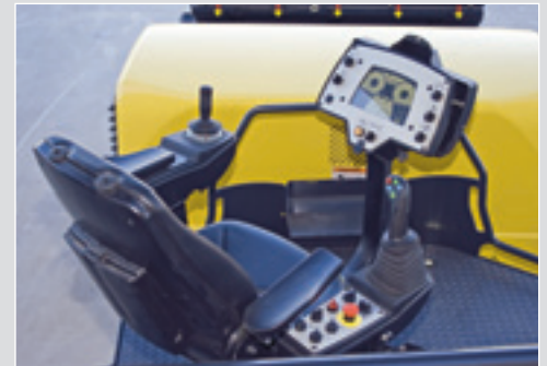
Joystick control travel direction, speed, steering, manual vibration on/off and MSP1 input from either seating position.
