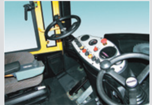
Two steering positions with a swivel/sliding seat makes the work environment more comfortable and safe.
