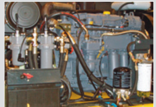
The engine: Rear, transverse positioned for ease of access and maintenance.
