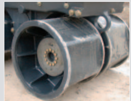
Optional Polygonal drum design offers increased compaction performance and machine gradeability.
