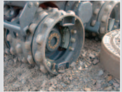
Bolt-on drum extension (std.) increases compactor versatility.
