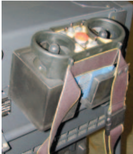
Removable operating console with cable remote control as standard
