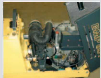
Power in reserve under severe conditions with the high torque 2 cylinder Hatz diesel engine
