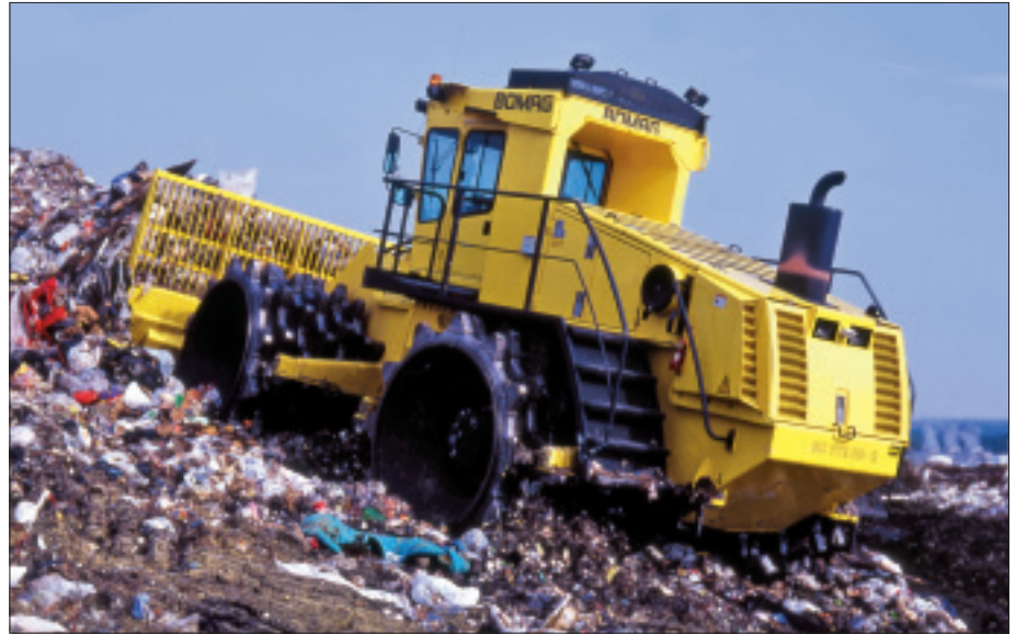
4-wheel hydrostatic drive system is capable of 100% gradeability, 45° slopes
