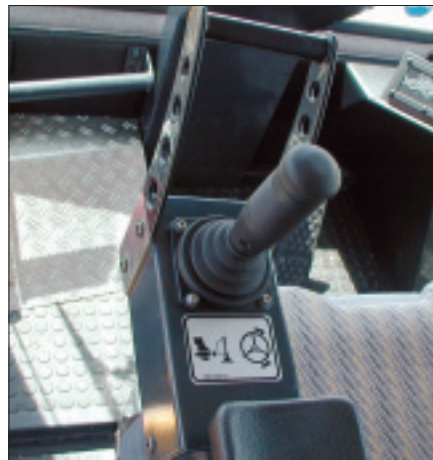
Ergonomic control layout including joystick steering control.
