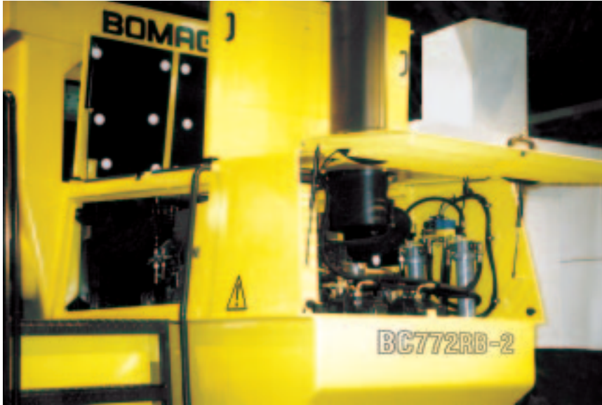
Easy access to the engine compartment through hinged doors.
