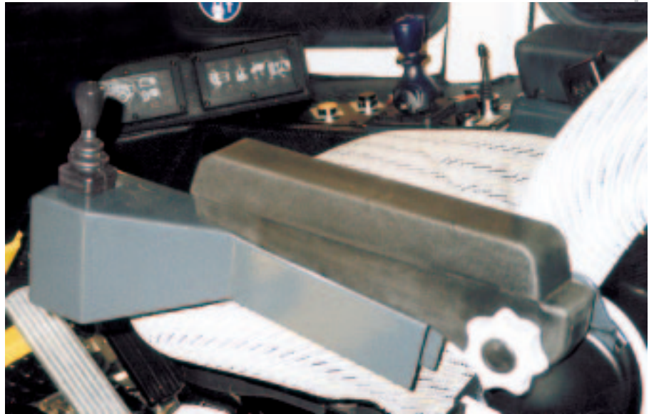
Ergonomic control layout including joystick steering control.
