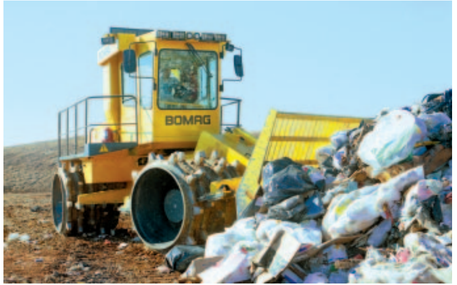
The operator's cab is vibration-isolated with excellent all-around visibility
